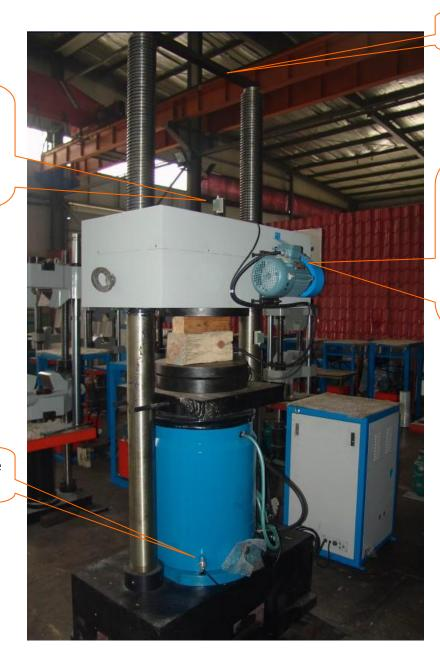
Worm wear and worm wheel structure: an electric motor drives the crosshead to move up and down
